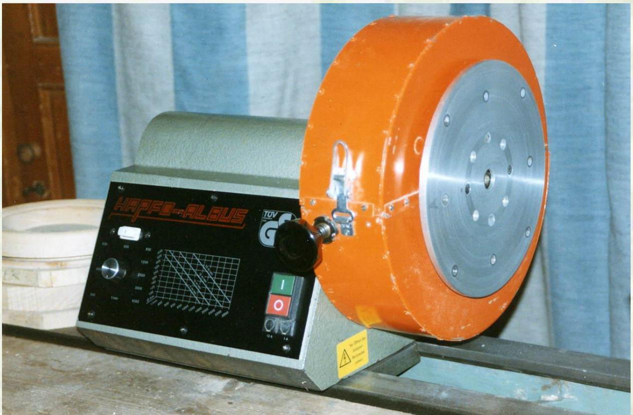
Figure 3403 Ovalturning Lathe ODM30
