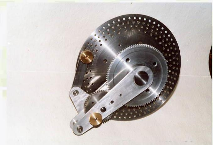
Holtzapffel [1.2.1] describes the „Compensating Index“ as an Indexer. This ingenious but probably empirically dimensioned mechanism was invented around 1830. A kinematic analysis [1.2.5] has shown that this indexer could be substantially improved. Hence the „Improved Compensating Index“ (ICI) has been constructed as indexer for the classic oval
