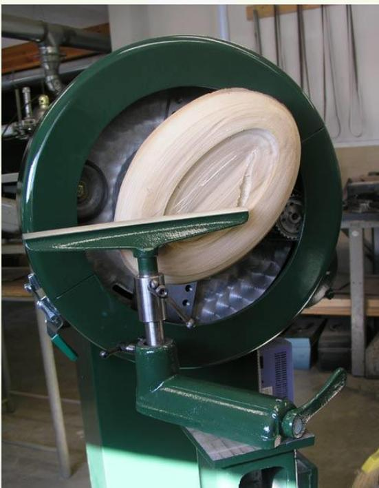
Dan [Bollinger](#), USA, has built a complete Ovalturning Lathe with a variant of the Volmer ellipse mechanism. Its maximum ellipse axes difference (sway) is very large. Other ovalturning devices using the Volmer Ellipse-Mechanism known to the author are shop-made by Buddy Lawson (Republic of South Africa), John Morgan (Australia) and Frank Freude (Germany).
