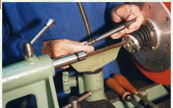
Pull out the ball-pin using the extractor (workshop J. Volmer) and enlarge the hole to fit the tang, saw off the spigot and sand the elliptical end round.
